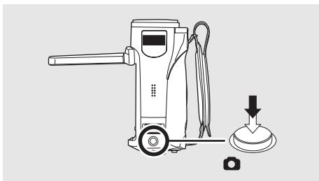
The shutter speed and the iris/gain value are fixed and the unit focuses on the subject automatically.
