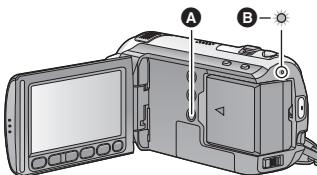
Press the power button **A** to turn on the power.
